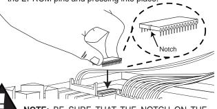
NOTE: BE SURE THAT THE NOTCH ON THE EPROM ALIGNS WITH THE NOTCH IN THE EPROM BASE.
