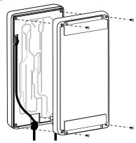
NOTE: IF THE KEYPAD BRACKETS ARE COVERING THE SCREW HOLES, REMOVE THE BRACKETS FIRST AND THEN REMOVE THE KEYPAD SCREWS.
