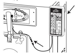
Remove the cabinet top by loosening the 6 screws along each side and partially lifting the front end to access the power supply cable harness on the electronics board.
