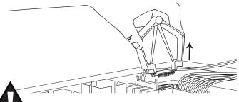
NOTE: HANDLE WITH CARE -- EPROM PINS MUST REMAIN UNIFORM! RETURN THE ORIGINAL EPROM WITH THE PACKAGING FROM THE UPDATED EPROM TO ENSURE PROPER CREDIT.
