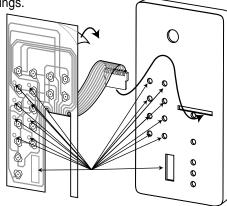
Remove the protective tape from the back of the small label strip and affix it to the exposed section of the keypad face under the ribbon slot. Ensure the circles on the label strip line up with the keypad panel's circular openings.
