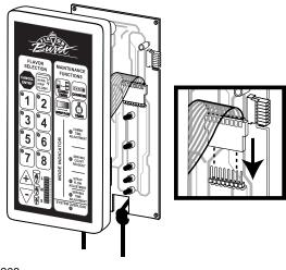
Line up the screw holes of the front cover, the electronics board and the back cover and secure them together with the screws. If the keypad brackets were removed, install them to the back of the keypad.
