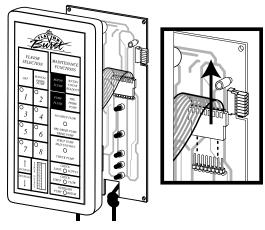
Use a flat head screwdriver to peel off a corner of the keypad label, then carefully remove the whole label and the switch membrane with ribbon behind it.
