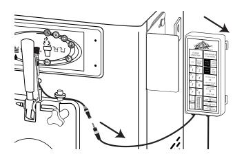
Loosen the outer screws and remove the back cover of the keypad.
