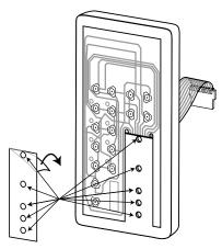
Remove the protective tape from the back of the new overlay keypad label and affix it to the face of the keypad face on top of the switch membrane. Ensure the transparent windows of the label line up with the keypad panel's openings.
