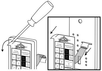
Remove the protective tape from the back of the ELE 523 switch membrane. Insert the ribbon into the slot on the keypad and affix the switch membrane to the keypad face. First ensure the rectangular opening on the switch membrane lines up with the opening on the keypad and then line up the 8 circles with the keypad's circular openings.
