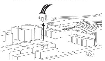
Using an EPROM pulling tool, carefully remove the existing EPROM in a vertical motion from the board.
