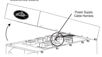
Disconnect the power supply cable harness to gain full access to the EPROM on the electronics board.
