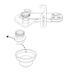
Install the modified Blending Auger over the Auger axis and work it in place so that the teeth of the Auger catch the gear of the Blending Assembly. Install the Hopper onto the Blending Assembly.
