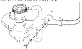
REV042110 pg. 1 of 2 Hang the suspension bracket on the lower door post and install the Blending Head onto the door spout. Install the Blending Head collar fully over the spout adapter and rotate the locking collar to secure.
