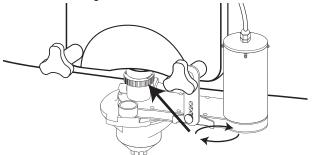
Use the Gear Box thumb nut to adjust the suspension bracket horizontally so that it hangs straight down from the door nut. Also, use the bracket thumb screw to adjust the bracket vertically so that it supports the Blending Assembly in a level position.
