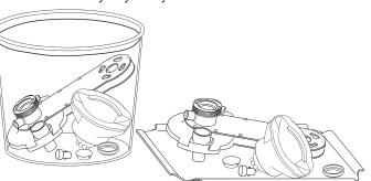
Place the seal in the Blending Auger and then place the Auger inside the Blending Hopper. Place the Auger and Hopper over the Blending Auger axis and into the grooves on the underside of the CW 172C Gear Box Assembly. Turn the Hopper clockwise until motion stops.
