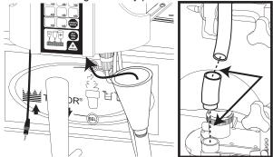
Remove the syrup port plug and insert the Flavor Burst 9-Tube Assembly manifold fully into the syrup port opening of the Blending Head. Rotate it until motion stops to secure the connection.
