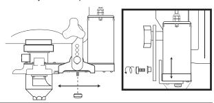
Install the top of the Hopper Tube Assembly into the Hopper opening until the Hopper Tube Adapter engages the lower portion of the internal Hopper funnel. Install the Tube Adapter and the lower end of the tube into the Blending Assembly port.
