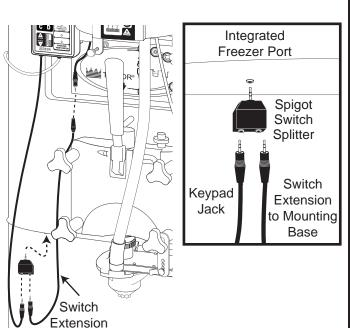
If the freezer uses a draw handle switch, connect the Switch Splitter to the switch. Plug the Keypad jack into one port on the Switch Splitter and the Mounting Base jack into the other port to complete the installation.
