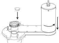
Remove the suspension bracket from the previous Gear Box Assembly and install it on the same side as the CW 172C Gear Box Assembly.
