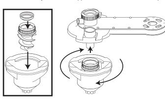
Insert the Drive Motor into the Gear Box so that all four locking screws are seated properly and rotate the Motor counter-clockwise to secure. Insert the hopper plug into the opening that will be closest to the freezer.
