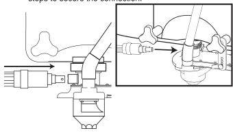
9A If the freezer has an integrated switch port, plug the Spigot Switch Splitter into the port. Connect the Keypad jack to one splitter port and the Switch Extension to the other port. Insert the Mounting Base jack into the port of the Switch Extension to complete the installation.
