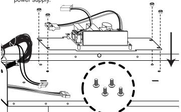
The new Power Supply should already have two cable connections attached to it. Connect the cable with the larger fitment to the Power Entrance Module fitment. Connect the smaller fitment to the Pump Harness Cable fitment.
