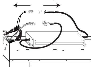
From inside the cabinet, unscrew the Power Supply from the locking nuts. Remove the Power Supply.
