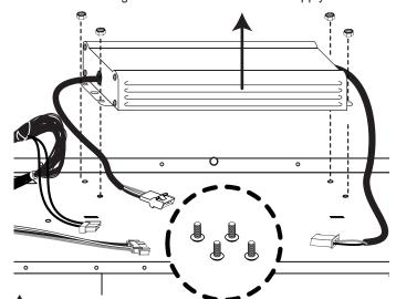
NOTE: FOUR SCREWS SECURE THE POWER SUPPLY FROM THE UNDERSIDE OF THE PANEL. YOU MAY NEED TO REMOVE THE TOP SYRUP TRAYS TO ACCESS AND REMOVE THE SCREWS.
