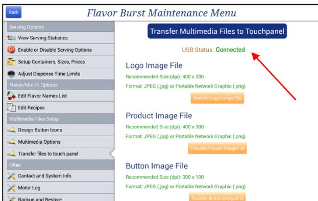
4. The five different TRANSFER buttons ensure the new files are uploaded from the thumb drive to the correct gallery folders. There are five different types of files you can upload: logos, product images, button images, background images, and videos. Upload each of your new files to the appropriate folders by selecting the corresponding TRANSFER button.
