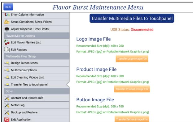
2. Load your new files onto a thumb drive. Ensure the files on your USB drive are PNG files or JPG files, and are the correct size for their purpose. Size (dpi) requirements are outlined on the screen.
