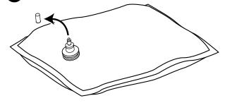
Lifting up the bag fitment, press the center pin of the fitment valve and gently press on the bag to release any excess air.
