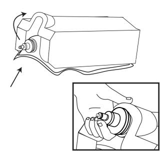
Holding the fitment in place, raise the open end of the tray and flip the tray right side up. As the tray is set back down, allow the bag to settle in the tray with the label
