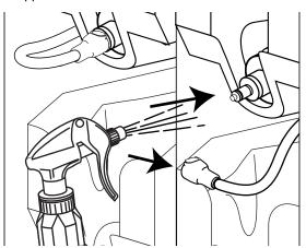
Connect the syrup bag connector to the bag fitment. Ensure the connector snaps and locks onto the fitment.
