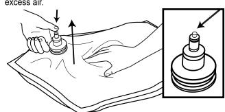
Place the tray up-side-down over the bag and pull the fitment into the tray opening as shown. The grooves of the bag fitment should slide into the tray opening.
