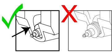
Install the syrup bag into a cabinet tray. Clean and sanitize the bag fitment and syrup bag connector with approved sanitizer solution.
