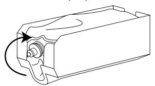
NOTE: DO NOT INSTALL THE SYRUP BAG FITMENT OVER THE TRAY SLOT. THIS CAN RESULT IN BREAKAGE OF THE FITMENT NOZZLE WHEN THE CABINET DOOR IS INSTALLED.
