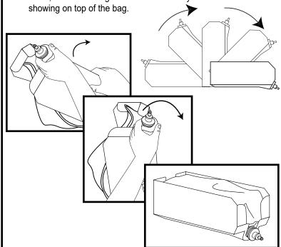
Lift the bag fitment out of the tray opening and set the fitment inside the tray cavity, behind the slot.
