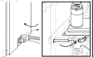
6 Spray the Syrup Bag Connector with sanitizer solution and allow it to sanitize for at least one minute.
