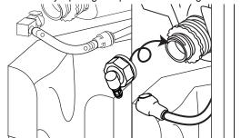
**NOTE:** IF STRAIGHT-VALVE SYRUP BAG ADAPTERS ARE ALREADY INSTALLED, REPLACE THEM WITH THE NEW ADAPTERS.
