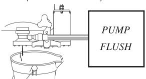
Press the ROTOR FLUSH key to clean the Injector Head.
