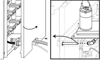
Remove the Syrup Tube Assembly from the cabinet.
