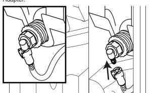
With a container under the Injector Head, press the numbered key corresponding to the syrup line (1-8) and then press the PUMP FLUSH key.
