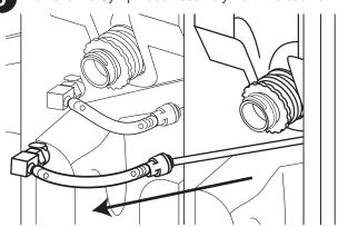
Slide the new SYR 945 Syrup Tube Assembly through the support railing to the back of the cabinet.
