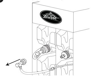
Slide the new SYR 944SH Syrup Tube Assembly through the support railing to the back of the cabinet.
