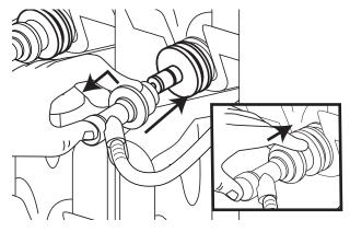
Place a container under the Blending Head, press the numbered key corresponding to the syrup line (1-8) and then press the WATER/SYRUP FLUSH key until the syrup line is fully primed. Press CANCEL ENTRY to stop the flush process once the syrup is flowing consistently.
