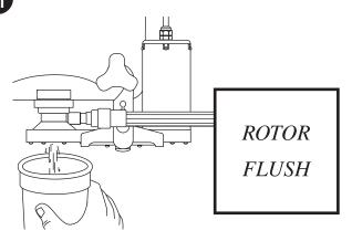
**NOTE:** FOR NEWER SYSTEMS, PRESS THE NUMBERED KEY CORRESPONDING TO THE SYRUP LINE AND THEN PRESS THE FLUSH KEY.
