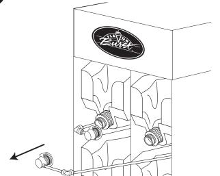
Slide the new SYR 944 Syrup Tube Assembly through the support railing to the back of the cabinet.
