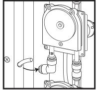
6 Spray the Syrup Bag Connector with sanitizer solution and allow it to sanitize for at least one minute.
