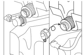
Hold the base of the adapter and turn the adapter valve toward the syrup line.
