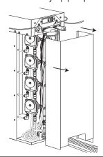
Remove the Syrup Tube Assembly from the cabinet.
