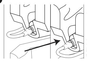
With a container under the Injector Head, press the numbered key corresponding to the syrup line (1-8) and then press the PUMP FLUSH key.
