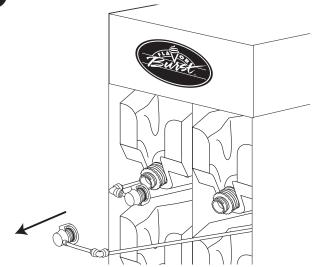
Slide the new SYR 944 Syrup Tube Assembly through the support railing to the back of the cabinet.
