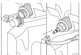
With a container under the Injector Head, prime the syrup pump by performing the PUMP FLUSH function for the syrup line.
