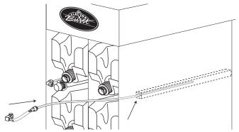
Insert the syrup tube fully into the elbow fitment of the syrup pump.
