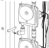
6 Spray the Syrup Bag Connector with sanitizer solution and allow it to sanitize for at least one minute.
