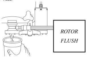
When cleaning the syrup line, remove the Syrup Bag Adapter from the bag fitment and install it on the Pump Flush Adapter. Then connect it to the Syrup Bag Connector and perform the Pump Flush procedure.
