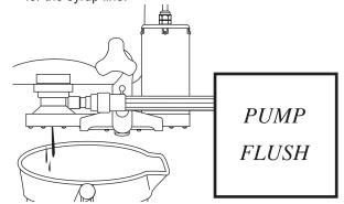
Press the ROTOR FLUSH key to clean the Injector Head.
