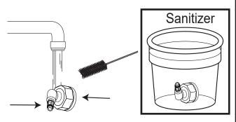
To clean the internal areas of the adapter, connect it to the Pump Flush Adapter (located under the bottom tray in the Flavor Burst cabinet). Place the Pump Flush Adapter over a container that is level with or below the sanitizer tank. Allow sanitizer solution to slowly flow through the adapter for 5 minutes.
