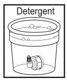
Brush and clean the adapter with the warm detergent water and then rinse thoroughly with warm water (108°F/42°C). Submerge the adapter in Stera-Sheen Green Label sanitizer solution for 5 minutes.
