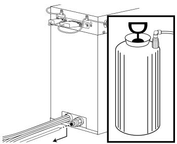
Fill the sanitizer tank with approved sanitizer solution. Install the cap and set the tank next to the cabinet.
