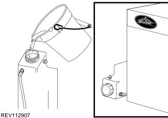
2 Connect the elbow fitment end of the sanitizer tank tube to the sanitizer fitment at the back of the cabinet. Connect the other end to the sanitizer tank connector.
