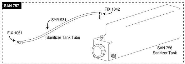
If the cabinet is connected to the older style sanitizer tank, disconnect the tank line from the connector at the back of the cabinet and remove the tank.
