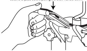
Continue to hold the Spigot Switch lever and pull the draw-handle down to dispense product.
