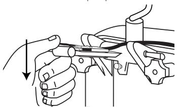
Just before the desired amount of product is dispensed, continue to hold the draw-handle down while releasing the Spigot Switch lever to stop the flavor flow to the
