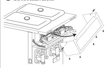
Loosen the two screws in the back of the display panel, then carefully pull the backing away from the display frame, making a gap.
