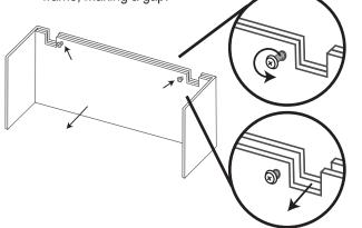
Slip the trans up between the backing and the diplay frame.
