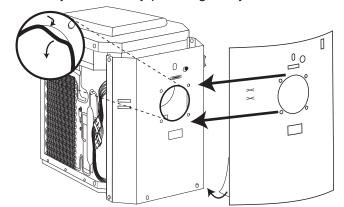
Line up the wrap with the panel underneath the power switch. Pull the two side light buttons through the "X" slits on the wrap, and fold the flaps to the inside of the panel.
