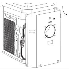
Remove the wrap backing and line up the large and small circular holes with the corresponding ones on the freezer. Roll back the black seal on the panel for the wrap to line up properly with the larger hole. Secure only this area by pressing firmly.
