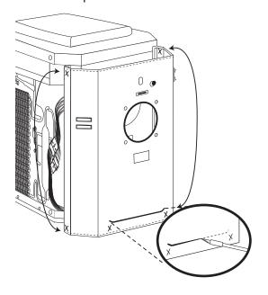
Make incisions where the wrap hangs over the panel corners and fold the wrap edges over onto the back. Press firmly into place.
