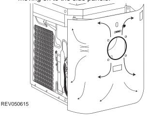
Remove the freezer face by carefully sliding it down and away, taking special note of the adjustment bolt. The face should remain attached to the freezer by wires. Set the face panel upright just infront of the freezer.
