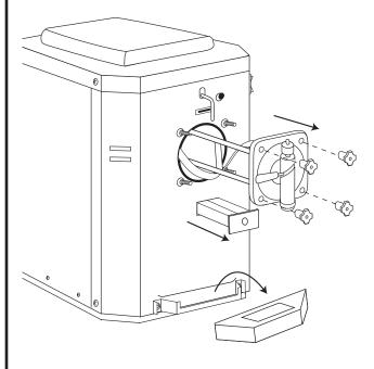
3 Using needle-nose pliers, remove the four screw pins from the freezer.
