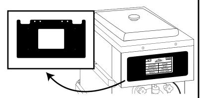
NOTE: NEVER APPLY THE WRAP TO THE TOUCHSCREEN PLATE OR USE A BLADE TO CUT THE WRAP WITH THE TOUCHSCREEN INSTALLED ON THE PLATE. THE ADHESIVE OF THE WRAP OR THE BLADE CAN DAMAGE THE SURFACE OF THE TOUCHSCREEN.
