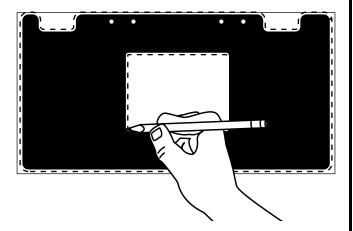
Carefully cut the wrap where marked. Score the wrap where it is marked for the screws.
