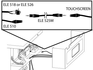
NOTE: WHEN CONNECTING TO A SWITCH WITH AN INSTALLED PANEL JACK SUCH AS THE ELE 518 AND ELE 526, THE CONNECTION CAN BE MADE OUTSIDE THE BOX. YOU MAY ALSO UNINSTALL THE JACK FROM THE DISPLAY FLOOR AND CONNECT IT TO THE TOUCHSCREEN PORT INSIDE THE DISPLAY BOX.
