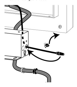
Connect the small power cable switch connection to the port at the far left of the electronics board.
