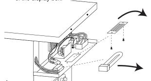
NOTE: WHEN INSTALLING ON A 432 FREEZER, REMOVE THE PLATE ABOVE THE SPOUT THAT HAS THE FLAVOR BURST ASSEMBLY INSTALLED. IF YOU HAVE ASSEMBLIES INSTALLED ON BOTH SPOUTS (I.E. TS 44BEV SYSTEM), REMOVE BOTH VENT PLATES.
