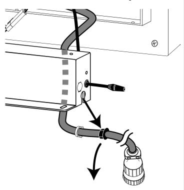
Pop out and completely remove the bushing holding the spigot switch port cable. Then push the cable back through the housing cover hole and away from the cover. Set the housing cover aside.
