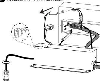
Leaving the rotor cable attached to the electronics board, pop out the strain relief bushing holding the cable. Slide the cable through the housing cover channel and away from the cover.
