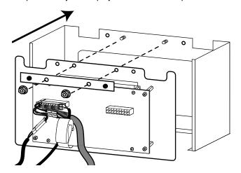
Insert the Touchscreen power cable and the Drive Motor cable through the vent opening of the display floor.
