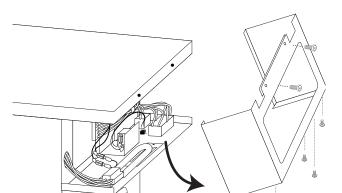
Remove the display box from the freezer.
