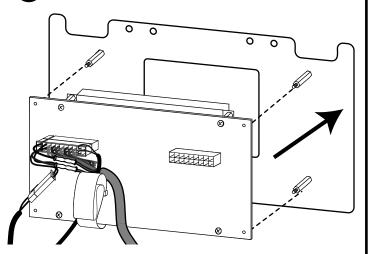
Secure the electronics board onto the spacer posts using the nuts provided.
