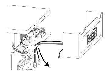
NOTE: IF YOU HAVE A TS 44BEV SYSTEM), INSERT A DRIVE MOTOR CABLE INTO EACH VENT OPENING. THE TOUCHSCREEN POWER CABLE SHOULD GO INTO THE OPENING CLOSEST TO THE SIDE WITH THE CABLE CASINGS.
