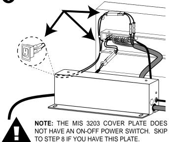
Carefully disconnect the switch from the Touchscreen electronics board and power cable.
