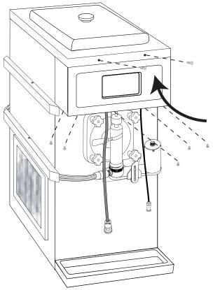
Reconnected the Touchscreen power cable and Drive Motor cable. Tuck excess cables inside the display box or hide them inside the cable casing. Cable ties and clips may be used to secure the cables underneath the display. Power up the freezer and Flavor Burst to complete the installation.
