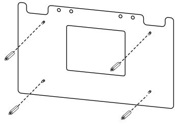
Install the electronics board onto the spacer posts.
