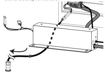
**9** Likewise, pop out the bushing holding the power cable and remove the cable from the housing cover.
