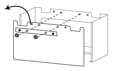
Install the electronics board and plate assembly to the display box in place of the plexi piece. Use the hardware provided by the display box to secure the pieces.
