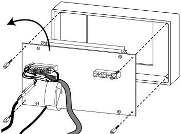
Screw the spacers onto the four posts of the Touchscreen display plate.
