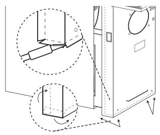
Two methods may be used to install the display panel trans, Slide the trans through the magnetic holder and then attch it to the display frame, or ...
