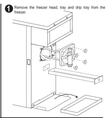
Using needle-nose pliers, remove the four screw pins from the freezer.
