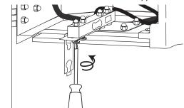
NOTE: DO NOT HOLD, LIFT OR PULL THE FAÇADE ASSEMBLY USING THE SUPPORT ARM OR THE WEIGHT SENSOR. THESE CONTAIN DELICATE ELECTRICAL CONNECTIONS. ALSO, DO NOT SET THE FAÇADE ON A SURFACE IN A WAY THAT PUTS PRESSURE ON THE SUPPORT ARM OR SENSOR.
