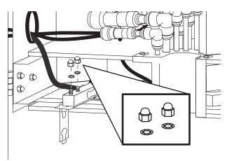
To tighten and secure the assembly, use a screwdriver to tighten the screws from underneath the support arm.
