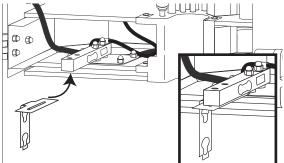
Use the two long screws to secure the support arm to the weight sensor. Screw them into the sensor all the way, with the ends coming up through the top of the sensor.
