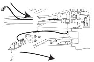
Attach the wire clamp around the wire of the new load cell approximately 3" from where the wire attaches to the load cell.
