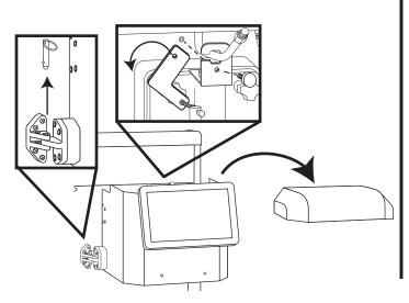
Swing the Door Assembly open and locate the load cell (weight sensor), attached to a mount plate at the lower
