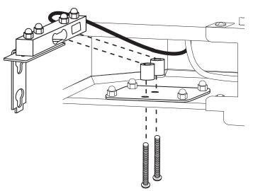
Disconnect the gland at the back of the cabinet labeled "WEIGHT SENSOR". Remove the gland from the cable.
