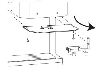
Open the Door Assembly by removing the lid, removing the latch pin, and disconnecting the lift bracket.
