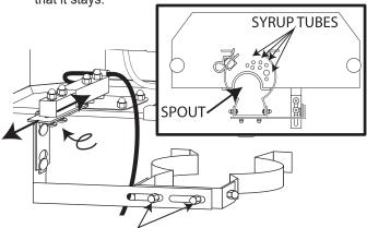
**NOTE**: THE NUTS ON THE CUP HOLDER ARM CAN BE LOOSENED IF IT IS NECESSARY TO ADJUST THE CUP HOLDER'S POSITION LEFT OR RIGHT.
