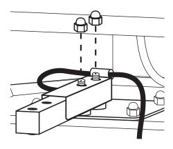
Remove the cup holder arm bracket with hardware from the old load cell. Install it on the new load cell in the same way, but do not tighten the screws all the way. The bracket should be able to slide back and forth for the next couple of steps.
