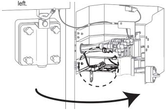
NOTE: THE LOAD CELL ON A CTP 80SNS-L SYSTEM WILL BE LOCATED AT THE LOWER RIGHT INSIDE THE DOOR ASSEMBLY.
