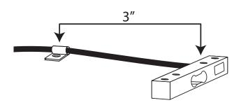
Using the two screws removed from the old load cell, thread the screws through the holes from underneath the Door Assembly and through the mount plate. Install the new (thin) spacer onto the screws. Then, install the new load cell onto the screws and spacers. Use the back holes nearest the cable, and position the load cell so that the cable to the far left side.
