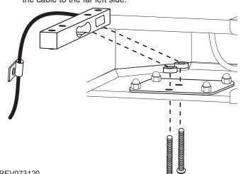
Install the wire clamp onto the furthest screw. Ensure the cable is perpendicular to the load cell where it is connected, and then curves around in a "U" shape.
