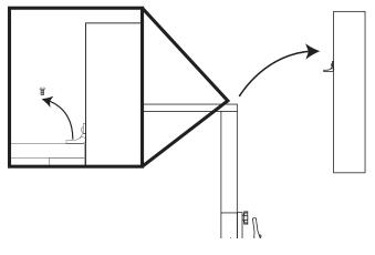
Line the bracket up flush with the top edge of the freezer and the lip of the bracket over the edge. Center it between the two notches on the bracket. Mark the freezer through the bracket screw holes.
