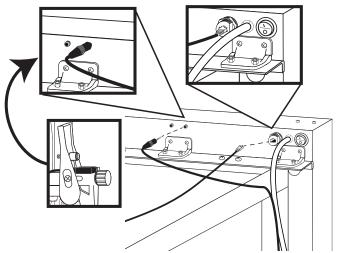
Remove the top panel of the freezer. Use the 4 screws to attach the bracket to the freezer and the nylon locking nuts to secure them from under the freezer panel.
