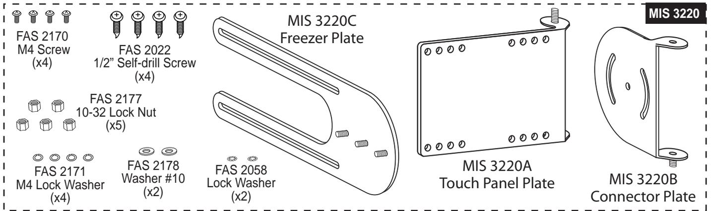
**1** Connect the Touch Panel Plate to the Connector Plate as shown, using two FAS 2177 lock nuts and FAS 2058 lock washers. Tighten the nuts just enough to hold the plates in position.
