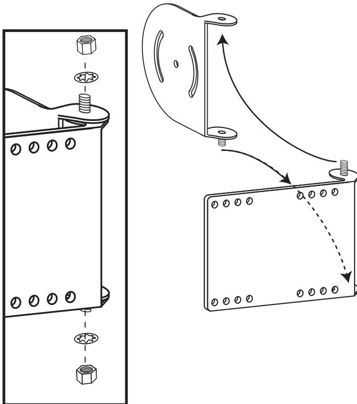
**2** Install the Touch Panel Plate to the back of the Color Touch Panel using the four FAS 2070 screws and FAS 2071 lock washers provided. When installing the Panel assembly on the right side of the freezer, the bracket hinge should be to the left. For left-side installation, attached the bracket on the Panel with the hinge to the right.
