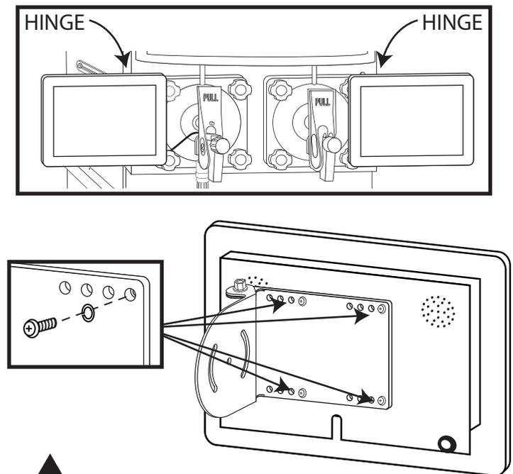
**NOTE:** THE CLOSER THE HINGES ARE TO THE OUTSIDE OF THE PANEL, THE LESS OVERHANG THERE WILL BE ON THE FREEZER. CHOOSE THE HOLE SET ON THE PANEL BRACKET THAT WORKS BEST FOR YOUR SETUP.
