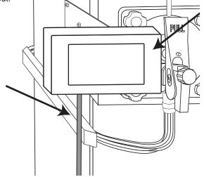
Arrage the bracket pieces into a configuration that will hold the Touchscreen in the chosen place against the freezer. All three plates can be flipped around depending on which side the Touchscreen is mounted. The connector plate has two sets of screw holes for the freezer plate, to move the Touchscreen closer or further from the freezer center.
