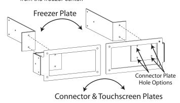
Remove the four corner screws on the back of the Touchscreen. Line up the mounting bracket assembly against the four corner holes of theTouchscreen, and secure it using the four screws.
