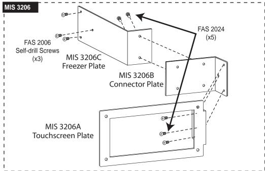
Connect the Connector Plate to the outside of the Touchscreen Plate using the three screws provided.
