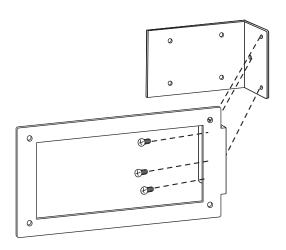
If you wish to angle the Touchscreen up or down, make the adjustment to the brackets and tighten the screws to secure the position.
