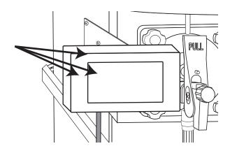
Open the Casing Assembly and place the Touchscreen cable inside. Close and secure the casing. Follow the Operations Manual to connect and power up the Touchscreen to complete the installation.
