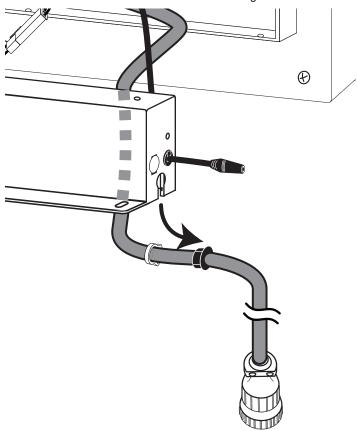
8 Pop out and completely remove the bushing holding the spigot switch port cable. Then push the cable back through the housing cover hole and away from the cover. Set the housing cover aside.
