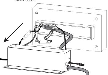
Locate the wires that connect to the power switch.
