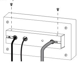
Slide the rotor cable through the left slot of the MIS 3203 cover plate. Insert the spigot switch port through the large middle hole. Slide the power cable through the cover slot on the right, in between the bushing and the
