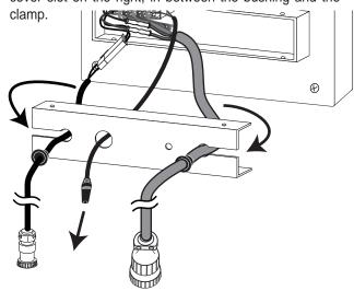
Place the new housing cover over the Touchscreen opening. Carefully guide the excess cable through each hole and pop in the bushings to secure the cables.
