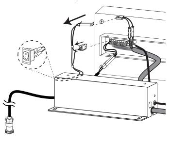
6 Leaving the rotor cable attached to the electronics board, pop out the strain relief bushing holding the cable. Slide the cable through the housing cover channel and away from the cover.
