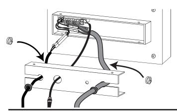
Using the screws from the old housing cover, install two screws to the top of the new cover to secure the assembly.
