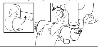
Swing the latch bracket down to close the bracket behind the Blending Assembly and around the door post to complete the assembly.
