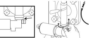
Install the Mounting Bracket over the Blending Assembly motor and onto the door post. Ensure the bracket hangs directly below the door post.
