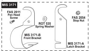
Assemble the Mounting Bracket as shown. Insert the screw through the large bracket plate, then through the spring washer and finally through the back plate. Secure the assembly with the nut and tighten.
