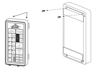
Attach the menu panel to the back of the keypad bracket using the nylon spacers and the FAS 2014 screws provided. Ensure the nylon spacers are installed between the menu panel and the keypad bracket, and tighten the screws. Proceed to the final step "Installing the Flavor Labels."
