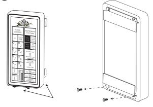
Attach the menu bracket to the back of the keypad bracket using the nylon spacers and the FAS 2014 screws provided. Ensure the nylon spacers are installed between the two brackets, and tighten the screws. Proceed to the final step "Installing the Flavor Labels."
