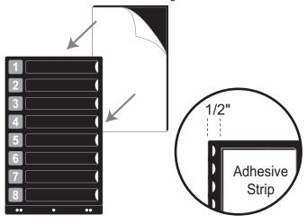
Remove the protective backing from the adhesive and press the menu panel assembly within the marks on the freezer. Proceed to the final step on page 2 "Installing the Flavor Labels."
