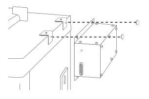
Ensure the power-switch is in the "off" position. Connect the Mounting Base Cable to the receptacle on the Electronics Controller Box and tighten the relief screws to secure.
