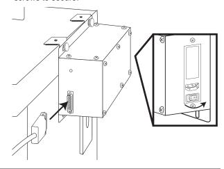
Connect the 110-volt (220-volt) power cord connector to the outlet on the Box and then plug the power cord into the wall receptacle to complete the installation.
