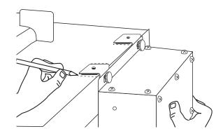
Install the two mounting bracket plates to the Electronics Controller Box and tighten each thumb screw to secure. The bracket can be configured into different positions to accommodate a vertical or horizontal mounting.
