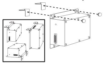
Remove the backets from the Box. Remove the protective tape from the adhesives and press each backet into place within the markings on the freezer. Allow the bracket adhesive to cure for at least 24 hours.
