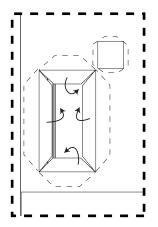
Slide the Keypad Cover over the Keypad to complete the assembly.
