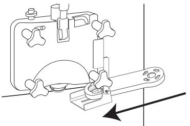
Install the Gear Cartridge and Injector Head onto the Gear Box and rotate the head to lock it in. Then attach the Injector Head to the spout adapter, rotating the metal ring over the adapter tabs to secure it.
