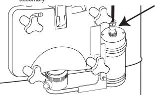
NOTE: TO REMOVE THE INJECTOR ASSEMBLY, LOOSEN THE GEAR BOX'S BOTTOM KNOB, REMOVE THE INJECTOR HEAD FROM THE SPOUT AND GEAR BOX, AND THEN LIFT AND SLIDE THE GEAR BOX ASSEMBLY OUT OF THE SUSPENSION BRACKET.
