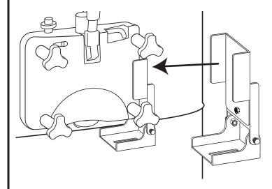
Slide the Door Bracket in between the freezer door and the
