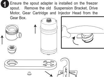
Determine to which side of the freezer the suspension bracket will be mounted. Assemble the bracket as shown. Only tighten the screws, nuts or knobs enough to hold the assembly together but are able to move the bracket parts.
