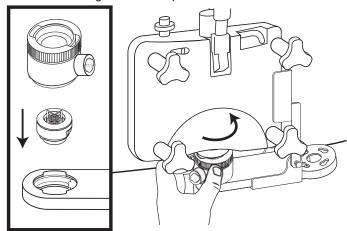
Position the bracket so that it is in-line vertically and horizontally and the Gear Box is level. Tighten the knobs, screws and nuts to that the assembly is secure. Install the Gear Box thumb nut underneath the Gear Box.
