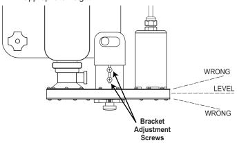
Replace the door hand screw and tighten to secure the Injector Assembly. Use the bracket screws for any
