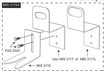
NOTE: TWO UPPER BRACKETS ARE INCLUDED WITH THE MIS 3119A SUSPENSION BRACKET ASSEMBLY. SELECT THE APPROPRIATE BRACKET FOR YOUR FREEZER: MIS 3117 (STANDARD) OR MIS 3117L (FOR MODELS WITH RECESSED HAND SCREWS).
