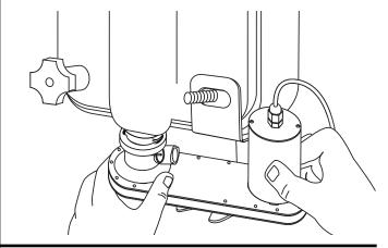
Ensure the Injector Assembly is level. If the Assembly is not level, adjust the screws on the bracket to the appropriate height.
