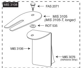
NOTE: THIS BRACKET IS OPTIONAL AND NOT INCLUDED AS STANDARD EQUIPMENT WITH THE FLAVOR BURST™ UNIT. BEFORE ATTACHING THE BRACKET, BE SURE TO THOROUGHLY CLEAN AND DRY THE FACE OF THE FREEZER WHERE THE BRACKET BASE WILL BE ATTACHED.
