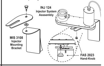
Ensure the INJ 124 Injector Assembly is level.
