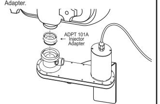
Move the bracket base into a position on the face of the freezer where the Injector Assembly is level. On the freezer panel, mark around the bottom and sides of the bracket base using a pencil.
