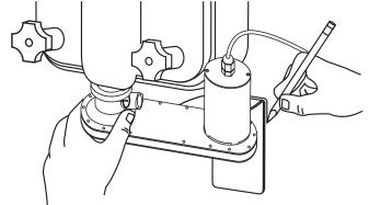
Assemble the bracket and attach it to the Injector Assembly using the black hand-knob.
