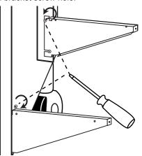
6 Ensure each bracket is level or perpendicular with the freezer side panel and make any necessary adjustments by loosening the bottom rail screw and adjusting the bracket until level. Tighten the screws to secure each bracket.
