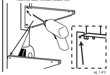
Install and tighten both FAS 2027 sheet metal screws into each bracket screw hole.
