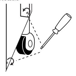
Slide each bracket groove onto each loosened screw and push the brackets inward as far as poissible. Tighten the screws to hold the brackets in place.
