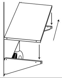
Install two FAS 2024 screws into the shelf lip and the front bracket and, if possible, two more screws into the shelf lip and rear bracket to complete the installation.
