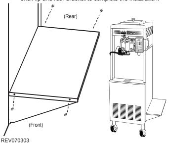
NOTE: IF THE SHELF EXTENDS OUT PAST THE REAR BRACKET, INSTALL THE TWO FAS 2024 FRONT SCREWS AND THEN INSTALL AN FAS 2024 SCREW INTO THE SIDE HOLE OF THE SHELF THAT ALIGNS WITH THE REAR BRACKET HOLE. TIGHTEN EACH SCREW TO SECURE AND COMPLETE THE INSTALLATION.
