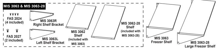
Choose which side of the freezer to install the shelf. Remove the freezer service panel and identify the right and left brackets. (The lips of each shelf bracket should face toward the inside of the assembly.)
