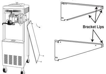
2 Locate both freezer rail screws inside the bottom of the opening. Back out each screw 2-3 turns, but do not remove the screws.
