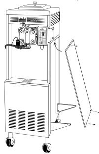
Position the shelf on top of the brackets and slide the shelf as far back to the rear of the freezer as possible.
