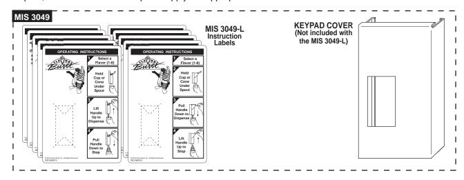
Peel the protective covering from the Keypad Cover and clean the surface before applying the label.
