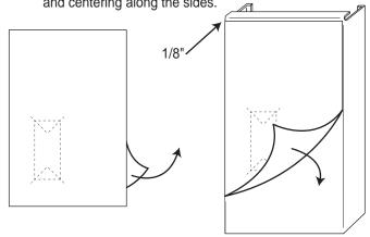
3 Cut along the dotted lines as shown and fold the edges of the label to the inside of the Keypad Cover openings.
