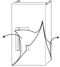
Remove the protective backing and apply the label to the Keypad Cover approximately 1/8" from the top edge and centering along the sides.
