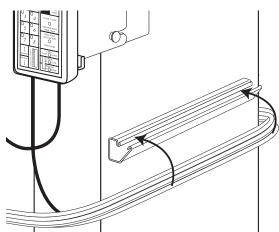
Close the Casing, and press all along the connection to secure.
