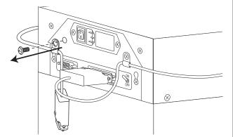
Wedge a screwdriver between the fold of the cable clamp and twist to open up the clamp. Remove the cable clamp from the cable.
