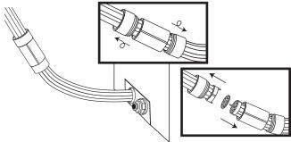
Connect the new 9-Tube Assembly to the Lead at the back of the unit according to instructions in the Operations Manual. Ensure the new 9-hole gasket is in place. (See EQUIPMENT SETUP "Syrup Line Unit Connection.")
