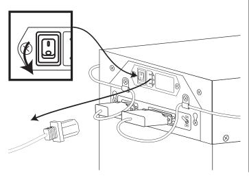
2 Loosen the 2 strain relief screws on the Rotor Motor cable connection and disconnect the Rotor Motor cable connection.
