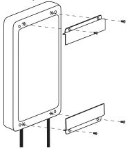
Remove the old Injector Assembly, Mounting Bracket, and Injector Adapter from the freezer door according to the old Operations Manual.
