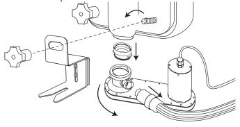
Assemble and install the new Injector Adapter, Mounting Bracket, Accessory Mounting Bracket, Keypad Bracket and Injector Assembly according to instructions in the new Operations Manual. EQUIPMENT SETUP for more information.)
