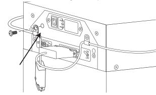
Connect the new Rotor Cable connection to the port on the back of the unit and secure by tightening the strain-relief screws.
