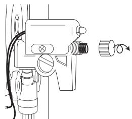
2 Insert the Flow Rate Controller inside the spring. Ensure the encased end of the assembly is toward the back of the spout.
