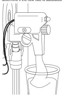
Adjust the Flow Rate Controller as needed. Adjust the screw further into the casing (shorten the assembly) to increase the flow rate. Adjust the screw out from the casing (lengthen the assembly) to decrease the flow rate.
