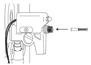
Install the door spout cap and draw a serving to determine if the flow rate is satisfactory.
