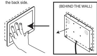
From behind the wall, place the right and left stabilizer brackets to each side of the Touch Panel as shown. Align all the slots of the brackets with the screw holes of the Touch Panel.
