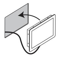
From this point forward, apply gentle pressure to the front of the Panel. If needed, use a partner to keep the screen in place while the brackets are being attached to
