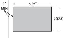
Place the Panel and any cords attached to it through the opening.
