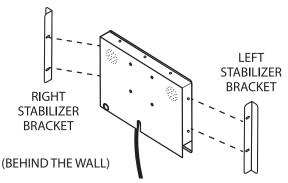
Install two hex bolts to each side of the Touch Panel to secure the stabilizer brackets. Gently press each bracket against the facade surface as you tighten the bolts. There should be no space between the front of the Touch Panel and the wall, or betweeen the wall and the brackets. Connect and install the CTP system as instructed in the Operations Manual.
