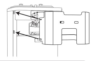
With a container under the spout, move the draw handle into the open position. If it comes in contact with the facade, loosen the support bracket hand knobs and adjust the facade until the draw handle is clear of it.
