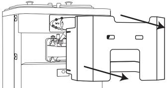
WARNING: DO NOT ADD CONSTANT WEIGHT, SUCH AS THE FACADE, TO THE BRACKETS BEFORE THEY HAVE CURED FOR <u>AT LEAST AN HOUR</u>. ADDING WEIGHT PULLS THE ADHESIVE STRIP FROM THE SURFACE AND IT WILL NOT ADHERE PROPERLY.
