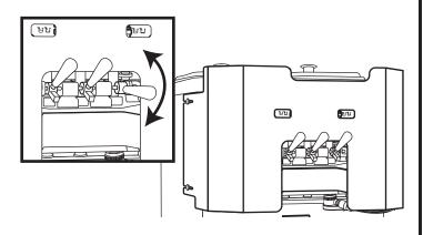
Remove the facade from the freezer so that the adhesive on the brackets can cure for <u>AT LEAST 1 HOUR.</u>
