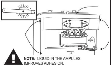
Measure and mark the each side of the edge of the freezer 1-3/4" down from the top, and then again 10-3/4" from the top. Make the marks from the edge of the freezer to the seam of the side panel. These mark the positions for the four side brackets.
