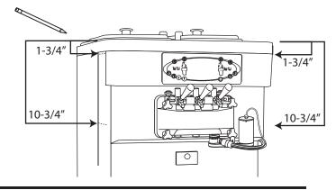
Remove the protective tape from each of the support brackets. Apply a bracket directly <u>under</u> each mark on the side of the freezer, as close to the service panel seam as possible without overlapping.
