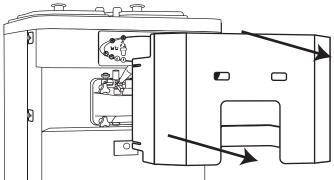
WARNING: DO NOT ADD CONSTANT WEIGHT, SUCH AS THE FACADE, TO THE BRACKETS BEFORE THEY HAVE CURED FOR <u>AT LEAST AN HOUR</u>. ADDING WEIGHT PULLS THE ADHESIVE STRIP FROM THE SURFACE AND IT WILL NOT ADHERE PROPERLY.
