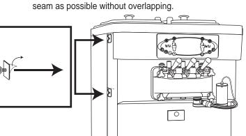
6 Install the facade onto the support bracket posts and secure it with the knobs.
