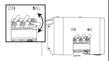
Remove the facade from the freezer so that the adhesive on the brackets can cure for <u>AT LEAST 1 HOUR.</u>
