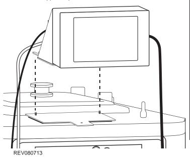
Secure the assembly to the base using the thumb knobs. Install the center thumb screw through the plate slot and the base screw hole.
