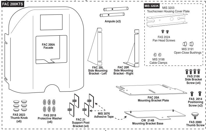
Remove the Flavor Burst Touch Screen, Touch Screen mounting brackets & plates, and the two metal cable/tube casings.
