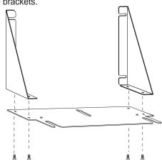
Remove the four corner screws from the back of the Touchscreen. Line up the side bracket slots with the screw holes. Secure the side brackets to the Touchscreen using the Touchscreen screws.
