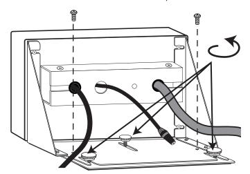
Twist the positioning screws in further until the Touchscreen is centered within the facade opening. Tighten down the thumb knobs and thumb screw to secure the position.
