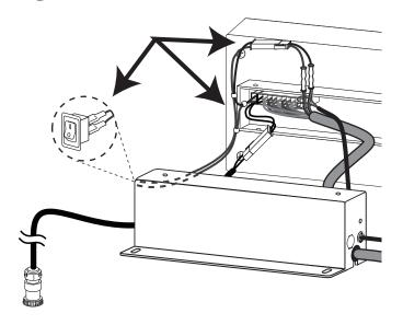
Carefully disconnect the switch from the Touchscreen electronics board and power cable.
