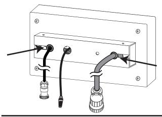
Using the screws from the old housing cover, install two screws to the top of the new cover to secure the assembly.
