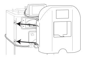
Ensure the Touchscreen opening lines up center with, or slightly above, the screen. If the opening falls below the screen, measure the distance needed to raise the facade until it is level. *Immediately* remove the support brackets, and raise them that same distance. Reinstall the facade to check the alignment.
