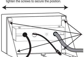
Reinstall the cable/tube casing and reconnect the Touchscreen cables to complete the installation.
