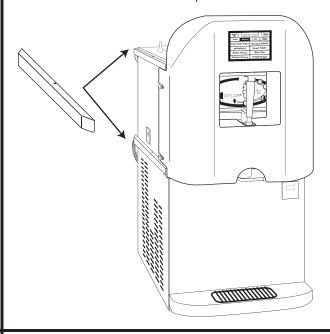
Once the touchscreen, mounting bracket assembly, and support brackets are in the proper positions, <u>REMOVE THE FACADE AND TOUCHSCREEN, AND ALLOW THE ADHESIVE STRIPS TO CURE FOR AT LEAST AN HOUR BEFORE REINSTALLING.</u>
