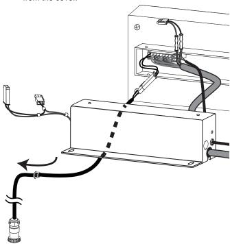
Likewise, pop out the bushing holding the power cable and remove the cable from the housing cover.
