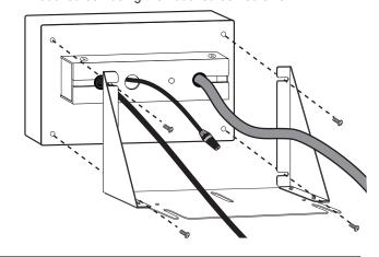
Install the Touchscreen assembly onto the mounting base posts and slide the assembly as far back towards the hopper as possible.
