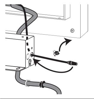
Connect the small power cable switch connection to the port at the far left of the electronics board.
