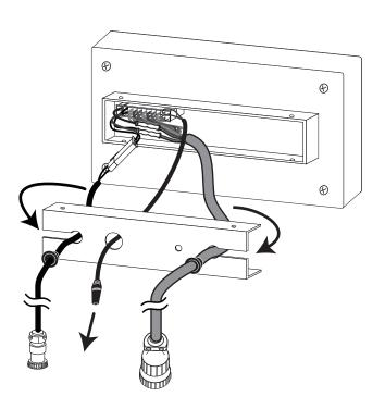
Install a clamp on the rotor cable on the inside of the cover near where the main cable splits. If your power cable does not already have a clamp, install one on it also.
