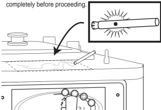
Apply primer ambules to the sides of the freezer, between the service panel seam on where the front surface begins to curve.
