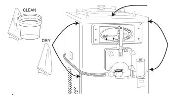
**NOTE**: THE FREEZER SURFACES <u>MUST BE</u> FREE OF ANY OILS OR RESIDUE OR THE ADHESIVE WILL NOT ADHERE PROPERLY.
