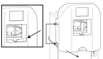
To slide the Touchscreen forward against the facade opening, loosen the center thumb screw and thumb knobs of the mounting bracket under the Touchscreen and move the Touchscreen forward. With the Touchscreen against the facade, tighten the thumb screw and knobs to secure the position.
