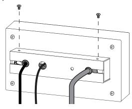
Install each side bracket to the mounting plate with the four flat head screws. Install the screws from underneath the mounting plate, and then up through the side brackets.
