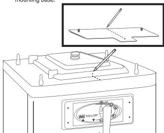
Remove the protective cover from the adhesive strip on the bottom of the mounting base. Line up the mark on the mounting base with the mark on the freezer and apply the plate to the freezer, as close to the hopper lid as possible. ALLOW ADHESIVE TO CURE FOR AT
