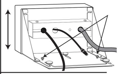
If the Touchscreen needs to be centered right or left within the facade opening, loosen the four corner screws on the back of the Touchscreen. Slide the Touchscreen right or left to center it within the opening, and then tighten the screws to secure the position.
