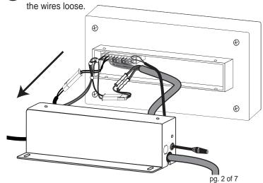
Q Locate the wires that connect to the power switch.
