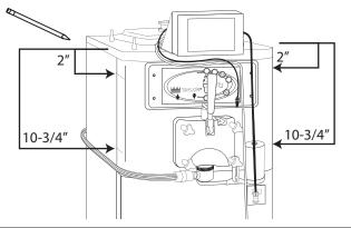
Remove the protective tape from each of the support brackets. Apply a bracket directly under each mark on the side of the freezer, as close to the curved edge as possible (approximately 1/4" from the service panel seam.
