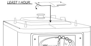
WARNING: DO NOT ADD WEIGHT, SUCH AS THE TOUCHSCREEN, TO THE BRACKET BEFORE IT HAS CURED FOR <u>AT LEAST AN HOUR</u>. DOING SO PULLS THE ADHESIVE STRIP FROM THE SURFACE AND IT WILL NOT ADHERE PROPERLY.
