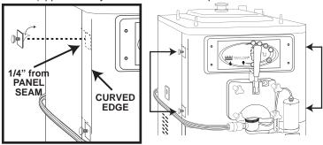
6 Install the facade onto the support bracket posts and secure it with the knobs.
