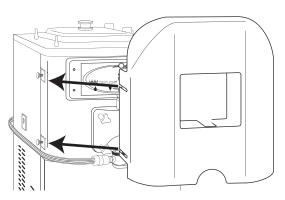
With a container under the spout, move the draw handle into the open position. If it comes in contact with the facade, loosen the support bracket hand knobs and pull the facade forward slightly until the draw handle is clear of it.
