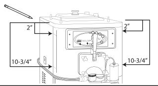
Remove the protective tape from each of the support brackets. Apply a bracket directly under each mark on the side of the freezer, as close to the curved edge as possible (approximately 1/4" from the service panel seam.
