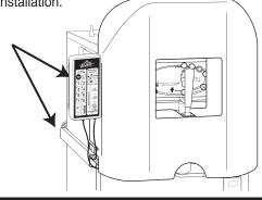
**OPTIONAL:** If your facade has a wrap, you can use the protective washers included in this kit to prevent the wrap from buckling and twisting when using the thumb knobs. Install the washer on the bracket post, between the knob and the facade.
