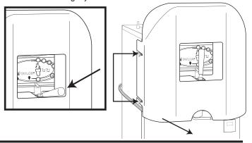
Once the support brackets and facade are in the proper position, <u>REMOVE THE FACADE AND ALLOW THE ADHESIVE STRIPS TO CURE FOR AT LEAST AN HOUR</u> BEFORE REINSTALLING THE FACADE.
