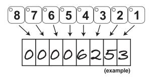
When all digits are recorded, press the COUNTER key to exit the mode. The resulting number is the number of servings the unit has dispensed since the last time the counter has been reset (example: 6,253 servings).
