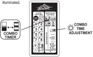
The number of illuminated bars in the graph represent the length of time each layer is dispensed. Use the following chart to determine the bar graph setting needed for the desired dispense time for each flavor layer.
