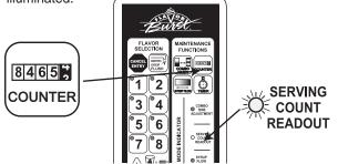
Select the #1 key and record the number of bars that illuminate on the bar graph as the last digit in the serving count. 10 illuminated bars on the graph represent "0"
