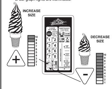
Press the TIMER key to exit the mode and lock in the setting. Repeat this process for each serving size (small, medium and large) until the desired serving time
