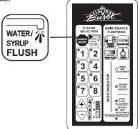
To prime a syrup pump or line, press the numbered key of the flavor. Then, press and hold the WATER / SYRUP FLUSH key for three seconds. Syrup will dispense for fifteen minutes before shutting off. Press CANCEL ENTRY at any time to stop the syrup flow
