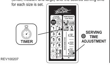
NOTE: WHEN A PARTICULAR SIZE IS SELECTED, THE SYRUP PUMP WILL STOP THE FLOW OF SYRUP AT THE SET TIME; TWO SECONDS LATER, A SOUND WILL NOTIFY THE OPERATOR TO CEASE DISPENSING THE SERVING. THIS ALLOWS SYRUP TO CLEAR THE INJECTOR HEAD, REDUCING CARRYOVER, AND INFORMS THE OPERATOR WHEN THE SERVING SIZE IS ACHIEVED FOR MORE CONSISTENT SERVING SIZE PROPORTIONS.
