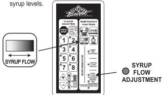
Draw a serving for each adjusted flavor to determine if the syrup concentration level is acceptable. Repeat this process for any flavors that need to be adjusted again.
