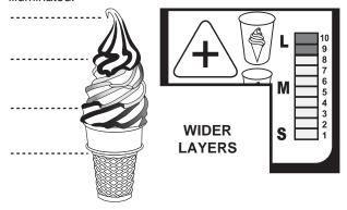
To decrease the timing (for more, narrower layers), press the "—" key until the correct number of bar graph lights are illuminated.
