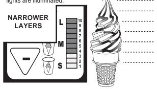
NOTE: IF THIS IS THE FIRST TIME THE COMBO TIMING HAS BEEN SET, SET THE TIMING TO ONE BAR (.5 SECONDS), DRAW A SERVING, AND ADJUST FOR WIDER LAYERS IF NEEDED.
