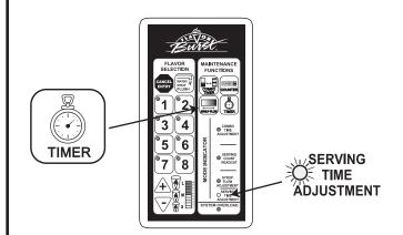
The number of illuminated bars in the graph represent the length of time the serving is dispensed. Use the following chart to determine the bar graph setting needed for the desired serving size time.
