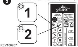
Press and hold the COUNTER key until there is an audible beep. After approximately 10 seconds, the registers will be cleared and the counter will be reset.
