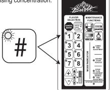
Press and hold the SYRUP FLOW key for three seconds until the SYRUP FLOW ADJUSTMENT light is illuminated.
