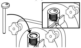
Place the switch assembly over the draw spout tube so that it is centered over the hole.
