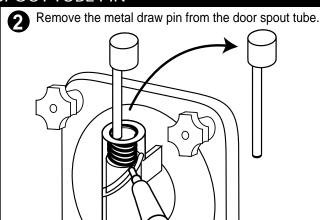
Insert the MIS 542A magnetic draw pin inside the spout tube so that it is flush with the top of the spout tube when the draw handle is in the open position.
