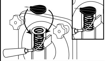
Connect the jack adapter to the switch, and the Keypad cable to the jack adapter to complete the installation.
