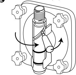
3 Place the magnetic actuator over the metal pin inside the door spout tube.
