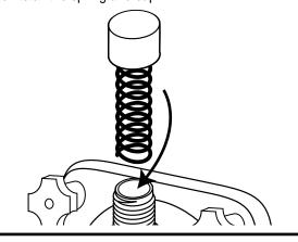
Place the switch assembly over the cap so that it is centered over the hole.
