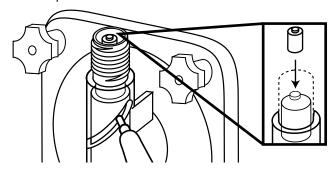
Return the draw handle to the closed position and reintstall the spring and cap.
