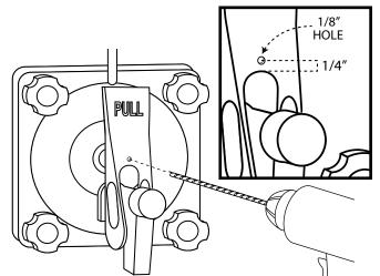
Attach the magnetic actuator to the front of hole using the bolt provided. Secure the assembly at the back with the nut as shown.
