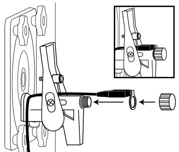
Connect the keypad to the switch. The magnetic pin activates the switch when the handle is pulled forward and the pin is brought close to the switch.
