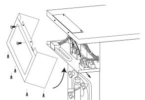
Replace the service side panel on the freezer to complete the assembly. Repeat instructions if installing another switch above the other freezer barrel on a Taylor 432.
