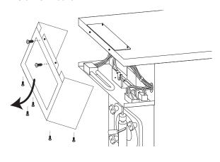
Attach the switch assembly just left of the Taylor internal switch, to the inside of the cover plate. The ELE 510 switch lever should be just above the internal draw pin as shown.
