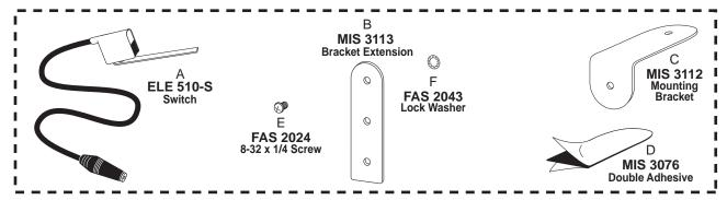
When possible, mount the ELE 510-S switch directly to the freezer without the bracket pieces. Bracket is provided if direct mounting is not possible.
