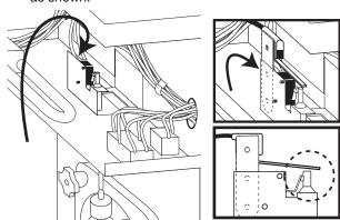
**NOTE**: THE SWITCH LEVER MUST BE FULLY DEPRESSED WHEN THE DRAW HANDLE IS IN THE OPEN POSITION.
