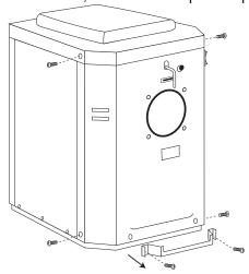
Remove the freezer face by carefully sliding it down and away, taking special note of the adjustment bolt. The face should remain attached to the freezer by wires as much as possible. Set the face panel upright just infront of the freezer.
