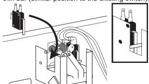
Line up the holes of the switch with the holes on the compartment wall. Install the two screws through the wall and switch, and secure them with the nuts.
