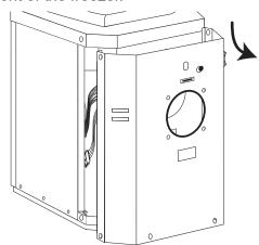
6 Locate the switch compartment on the inside of the freezer face, at the top center. You will see an existing switch inside the compartment area, and a space on the opposite side of the springs where the new switch will also be installed.
