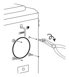
Unscrew and remove the tray bracket. Remove the freezer face screws located at the top and bottom of each side, near the side panel opening.
