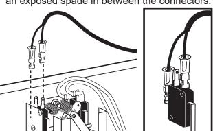
NOTE: Attach the spade connectors to the new switch to match the configuration of the freezer's existing switch. Depending on the model of freezer, this configuration may be different.
