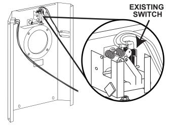
Place the new ELE 474-NCL switch inside the compartment wall, opposite the existing switch, with the two spades pointing up. The lever should be facing outward, angled downward, and pinned against the switch by a thin bar (similar position to the existing switch).
