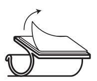
Attach the Retaining Clip to the underside of the ELE 447 Spigot Switch.
