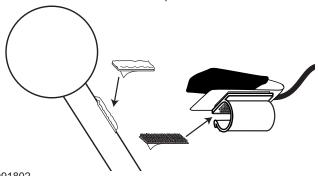
Be sure to align both sides of the Hook & Loop Tape as you rotate the Retainer Clip onto the draw-handle rod to complete the assembly.
