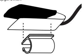
Rotate the Switch onto the draw-handle rod to complete the basic assembly.
