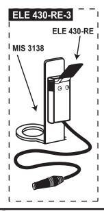
Remove the freezer handle and install the Switch Assembly over the exposed threads.
