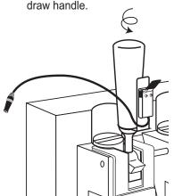
Be sure to fully engage the Spigot Switch jack to the Flavor Burst™ keypad jack for normal operation. Do not neglect to check this connection during daily startup.
