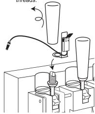
Replace the freezer handle and ensure that the Switch Assembly is the desired position as you secure the draw handle.
